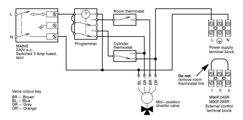
Fig. 6.19 - directly controlled boiler
