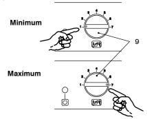
Fig. 2.9 Adjustment of the d.h.w. temperature is completely separate from that of the c.h. circuit.
