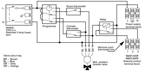
Fig. 6.18 - relay controlled boiler
